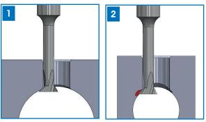
Is there an unfavorable ratio of the bore diameter between the longitudinal and the transverse bore, the risk of collision exists when deburring with a conventional cutting angle of 45  $^{\circ}$  (Figure 2, red zone).
