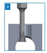
For deburring cutters with a cutting angle of 25  $^{\circ}$  there is no danger of collision.
