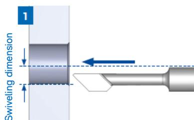
Position the central axis of the deburring tool on the center of the bore. Adjust the swiveling dimension so that the center of the deburring cutting edge meets the edge of the bore. The tool will be pressed to the axis against the spring force.
