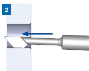
Immerse in the bore with rotating tool and large feed. The front edge of the tool is rounded to allow for easy immerse and to prevent damage to the outside bevel.
