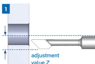
Position the central axis of the deburring tool on the center of the bore. Adjust the swiveling dimension so that the center of the deburring cutting edge meets the edge of the bore.
