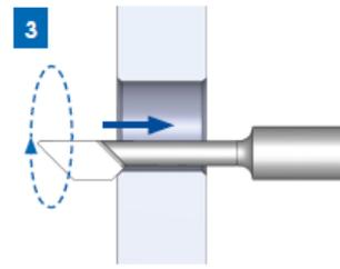
Only immerse until the tool swings outwards and the offset tool neck rests against the bore. Then drive backwards with a small feed, depending on the desired deburring intensity (about  $F=80$ ). In this process the burr will be removed because the blade is pressed by the spring force to the edge to be deburred. As soon as the cutting surface is clear, drive out of the bore with rapid-traverse.
