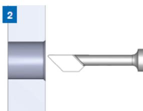
Adjust the spindle or workpiece in Z-direction so that the cutting edge can pass the hole without contact.
