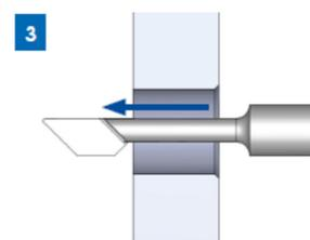
After adjustment, drive in rapid through the bore without rotation.
