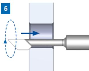
Switch on the rotation and drive slowly upwards until desired chamfer is reached.
