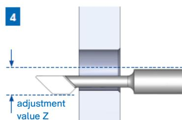
Then reset the spindle or the workpiece by the adjustment value.
